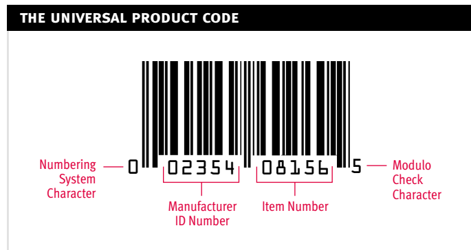
Figure 1. The Universal Product Code (UPC) is a numeric sequence representing manufacturer and product.
