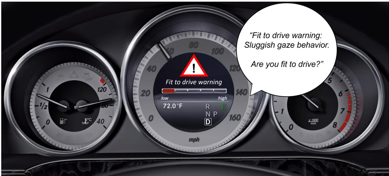
**Figure 12:** Example for a fit to drive intervention system. The system warns the driver with a visual- and audio-based intervention including a reason for the warning.
