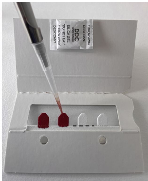
Figure 1. Design of the new volumetric filter paper cards (DBSV) with a paper comb with teeth and a perforation for detaching the teeth. The folding mechanism and the cover with a silica desiccant gel packet provide faster drying and protection of the samples during transport (a colored figure is provided online). The dashed line shows the perforation line where the teeth can be detached for the analysis.
