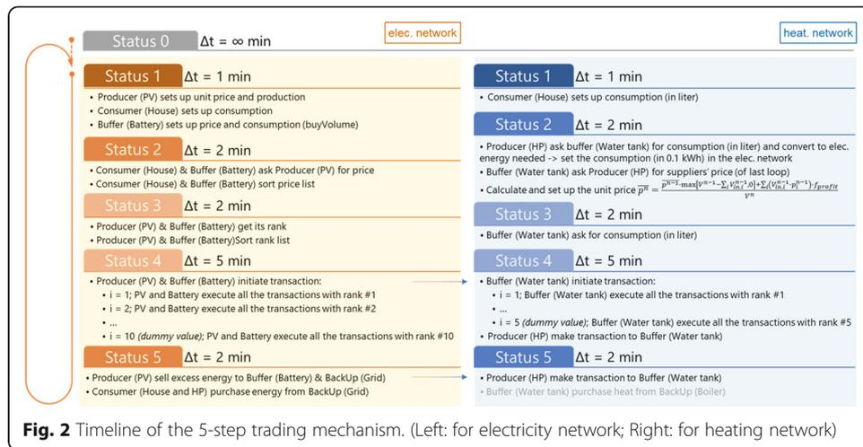
**Fig. 2** Timeline of the 5-step trading mechanism. (Left: for electricity network; Right: for heating network)
