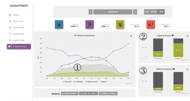
**Figure 11:** This screen shows a battery simulation available to a prosumer. The potential energy consumption covered by the battery is shown in the lighter green area (1). The bar graphs on the right show the differences with or without battery for self-sufficiency (2) and autarky (3).
