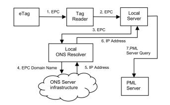
Fig. 3: A tag reader detects the EPC stored in the electronic tag and retrieves the network IP address of the associated PML server through a query of the ONS resolver, which then directs the request to the authoritative ONS server.
