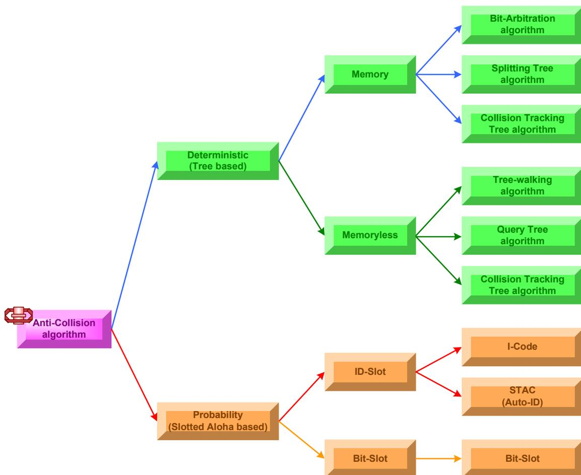
*Figure 5: Taxonomy of the existing tag anti-collision protocol*
