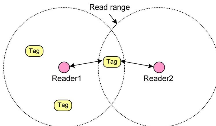
*Figure 3: Reader-to-tag interference*
