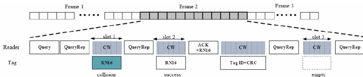
Figure 6: Multi-tag reply in EPC Class 1 Gen.2 Protocol
