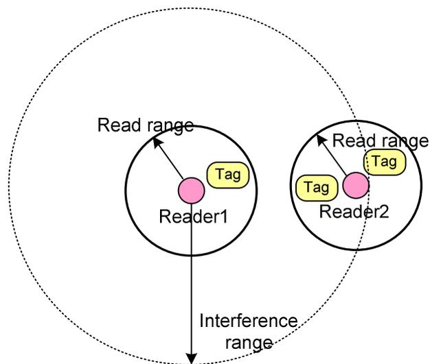
*Figure 4: Reader-to-reader interference*
