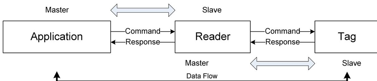
*Figure 1: A Master-Slave Principle in RFID Systems*
