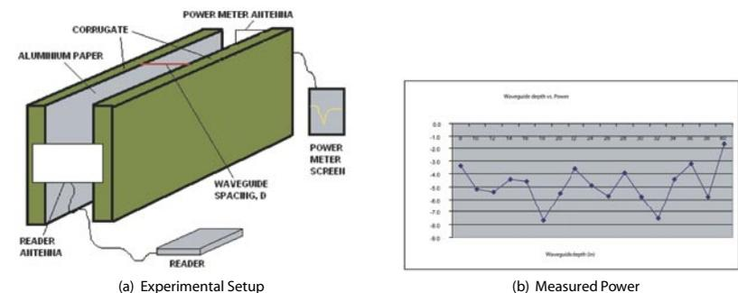
Figure 3: Waveguide: a packaging feature to improve tag readability
