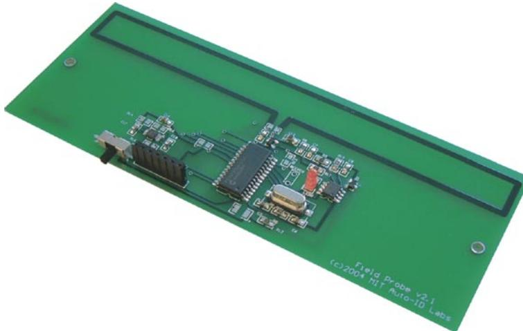
*Fig. 2: Field Probe: a semi-passive emulation tool*
