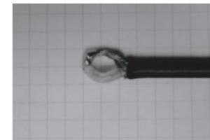
Fig. 5: A simple small loop used to determine resonance point of RFID tag
