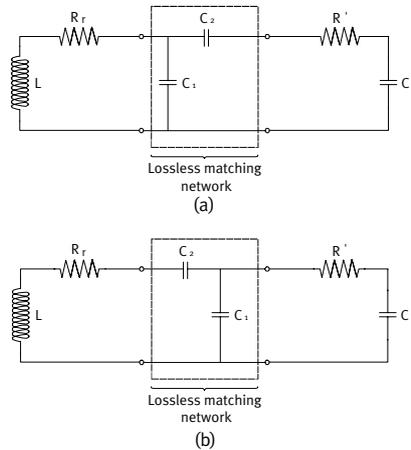
Fig. 3: (a) A lossless L-matching network with a shunt capacitor ( $C_1$ ) and series capacitor ( $C_2$ ) for matching; (b) Another lossless L-matching network with different arrangement of  $C_1$  and  $C_2$ .
