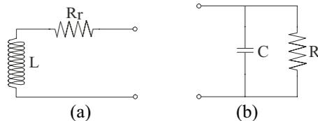
Fig. 2: Equivalent circuit for (a) a loop antenna; (b) RFID tag chip
