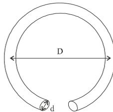
Fig. 1: The proposed loop antenna
