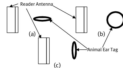
Fig. 6: Orientation of tag with respect to interrogating antenna: (a) Horizontal; (b) Vertical; (c) Parallel
