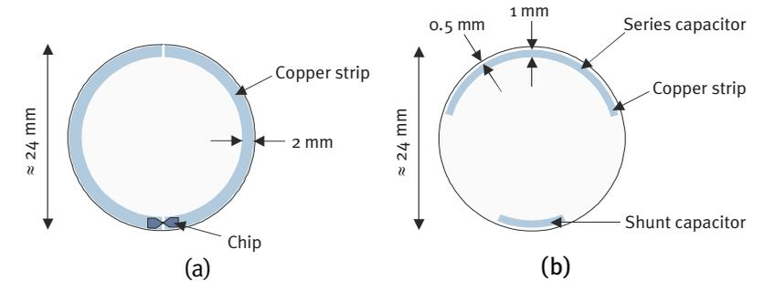
Fig. 4: (a) Front view; (b) Rear view of the sheep ear tag
