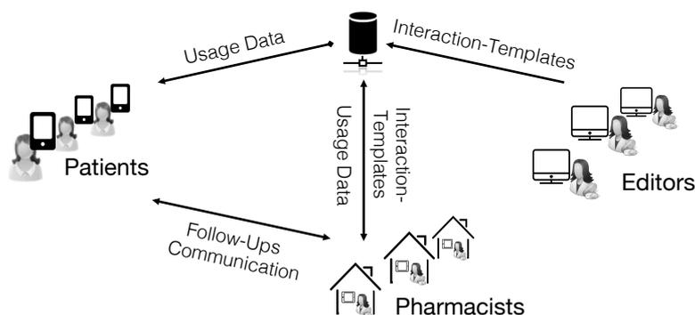
Figure 1. HIS Overview: tablet-PC-app for pharmacists, smartphone-app for patients, web-interface for editors, and a backend based on Titanium (<http://appcelerator.com>).
