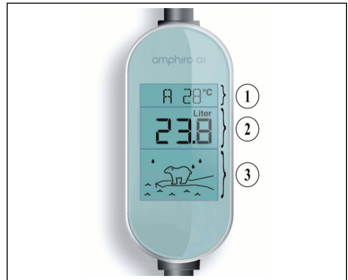
Figure 2: Amphiro shower smart meter showing the current energy efficiency class [rated from A to G], temperature [ ^{\circ} C], water volume [liters] and a polar bear animation. As soon as the water flow stops, water and energy consumption [(k)Wh] toggle.
