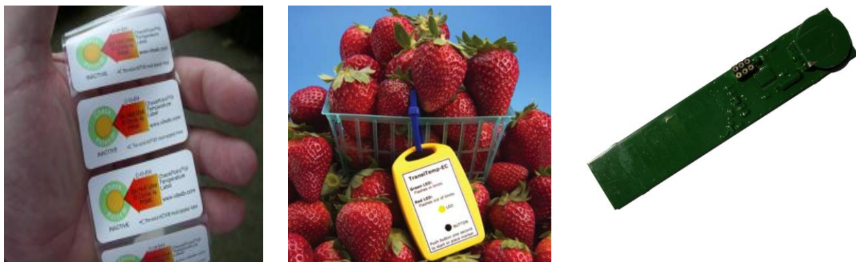
Figure 1. Different temperature tracking technologies: TTI label (source: Vitsab), data logger (source: MadgeTech), and a semi-passive RFID tag (source: Caen)
