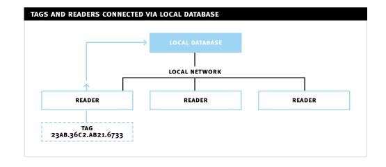
The most attractive way to network readers and sensors is through a TCP/IP network. However, TCP/IP controllers are expensive today. We are looking at other standards including RS 232 (implemented), RS 485 (implemented), Lon Works IEEE 1473 (under investigation). Issues being investigated include data rate, power requirements, wire-length considerations, and robustness.
