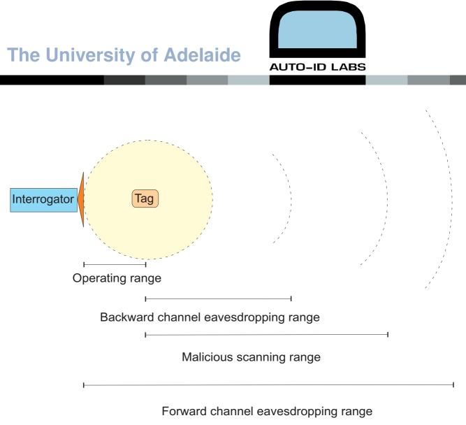
Fig. 1: Tag reading range classification.
