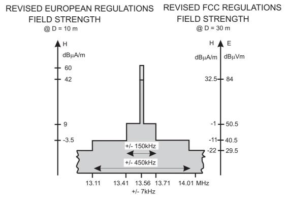
Fig. 3: HF electromagnetic compatibility regulations.
