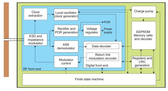
Fig. 1: Block diagram of a passive UHF/HF RFID label.
