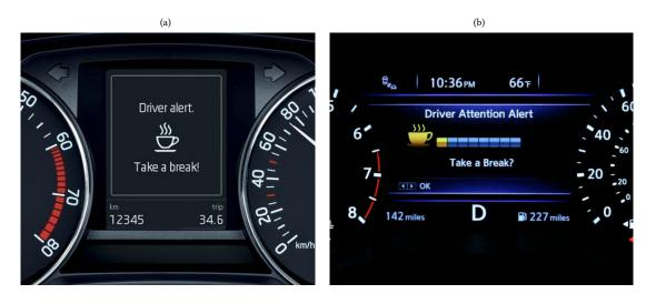
Figure 1: Examples of existing drowsiness and attention warning systems in today's cars. (a) Drowsiness warning delivered in Volkswagen cars; (b) Attention warning delivered in Nissan cars.
