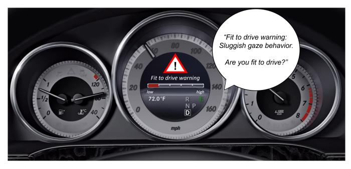
Figure 12: Example for a fit to drive intervention system. The system warns the driver with a visual- and audio-based intervention including a reason for the warning.
