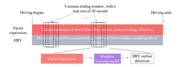
Fig. 5. HRV outlier detection framework
