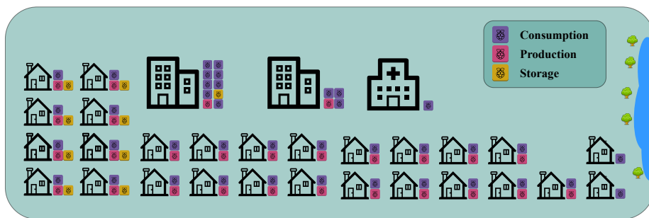
Figure 1: Setup of the Walenstadt microgrid. The district consists of 37 participants with varying configurations. Two apartment buildings, eight prosumers with local storage, seventeen prosumers, two consumer households, as well as an elderly home as a large consumer.
