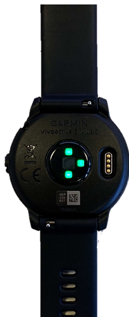
Figure 2: Back view of a consumer smartwatch with its optical pulse sensor active (green LEDs).
