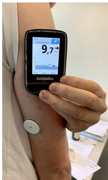
Figure 1: A person with an invasive, continuous glucose monitor sensor in their upper arm and its corresponding reader.
