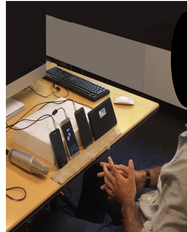
Fig. 7. Recording setup. Note: A computer screen was used to provide the instructions; the mobile devices were positioned with their microphones facing upwards; From left to right: NT1000, iPhone 5, Galaxy S5, One M8, and Nexus 7
