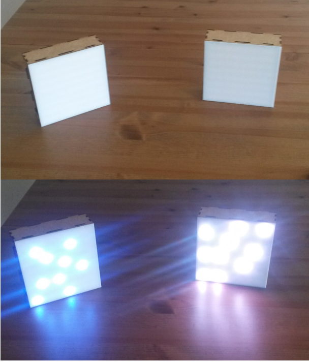
Fig. 2. The boards are packaged in a wooden box and LEDs are behind a semi-transparent screen. Top image shows in off state and bottom image with a few random LEDs in on state.
