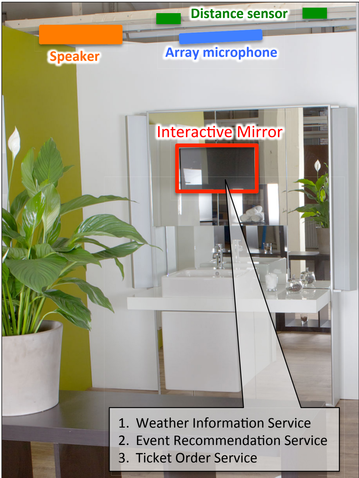
Figure 10. Three UIS services embedded in the mirror of the bathroom
