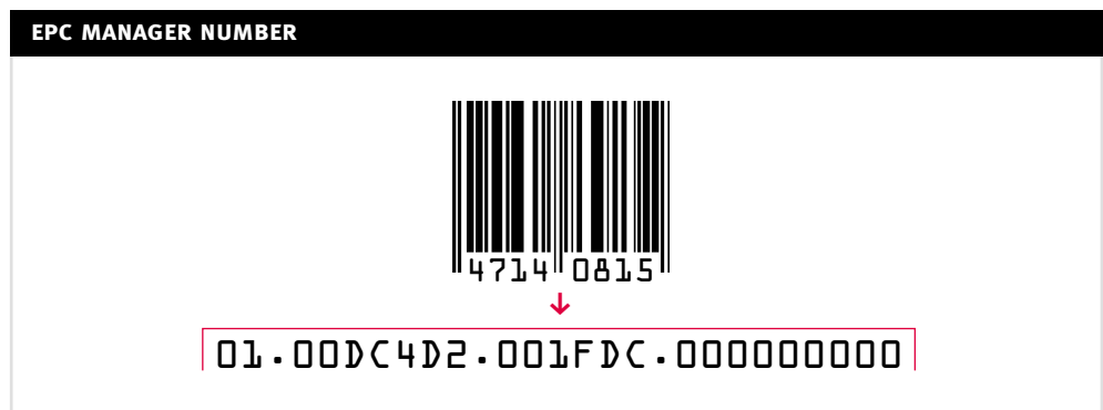
Figure 13. Adding an EAN/UCC Country Code specific offset to the EAN/UCC Manufacturer Identification Number forms the EPC Manager Number. The EPC Product Class and EAN/UCC item number are identical
