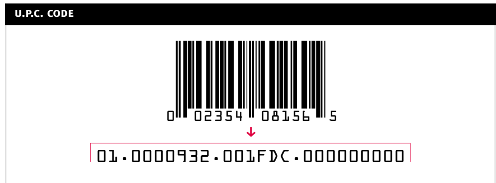
Figure 11. The manufacturer and item numbers of the U.P.C. code map directly into the manager and object class numbers of the EPC.
