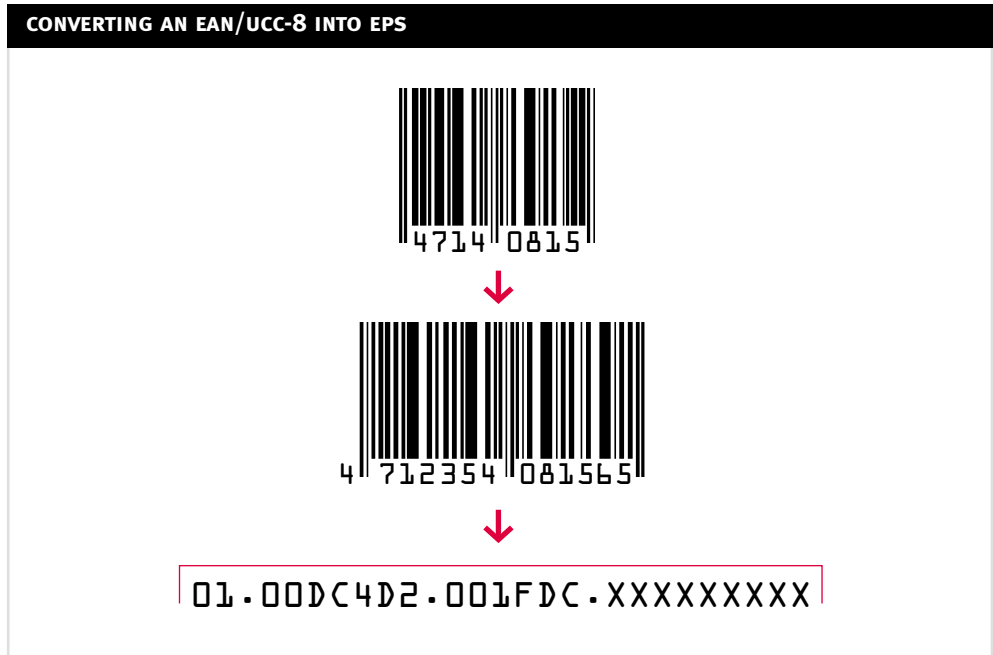
Figure B5. To convert an EAN/UCC-8 into an EPC, first convert the 8-digit code to the corresponding EAN/UCC-13 and then convert the 13-digit code to an EPC.
