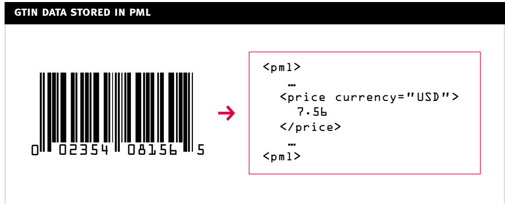
Figure B2. Data in the GTIN will be stored in Physical Markup Language (PML) data files. Here the $7.56 price for a random weight item is recorded as a value in the PML price element.
