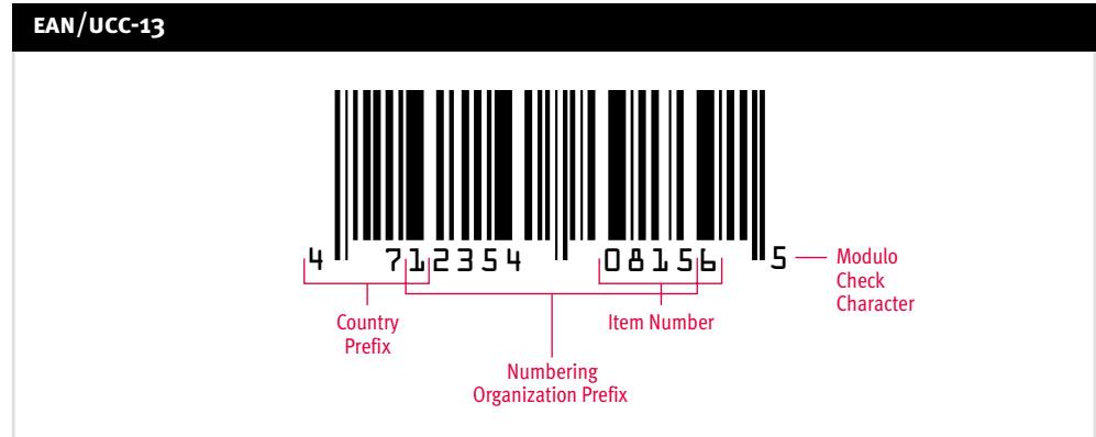
Figure 8. The EAN/UCC-13 is a 13-digit code used to identify product in sold in countries outside the United States and Canada.
