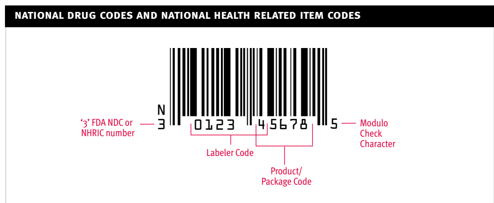
Figure 5. National Drug Codes (NDAC) and National Health Related Item Codes (NHRIC) are embedded in the UPC.
