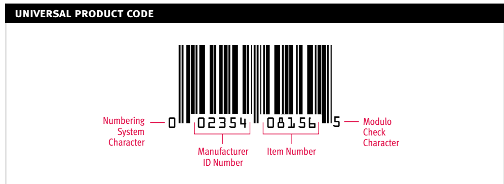
Figure 2. The Universal Product Code UCC-12 (U.P.C.) (UPC version A shown) is a numeric sequence representing numbering system, manufacturer, product and checksum.
