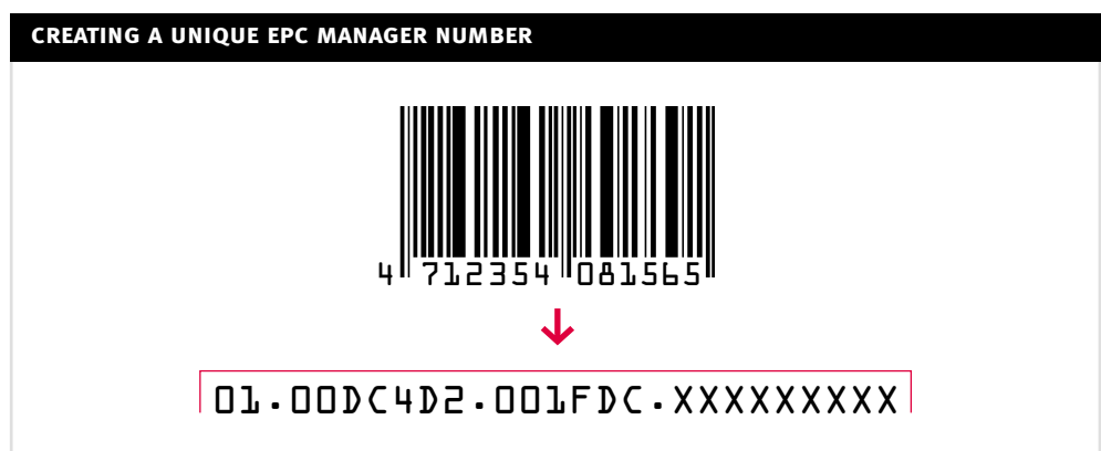
Figure B3. Adding an EAN/UCC Country Code specific offset to the EAN/UCC Manufacturer Identification Number forms the EPC Manager Number. The EPC Product Class and EAN/UCC item number are identical.
