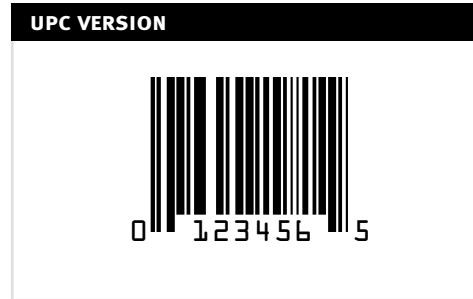
Figure 3. The UPC version E is a zero suppression version of the UPC and is intended to be used on packaging too small to accommodate the full version A. These are commonly seen on soda cans and bottles.
