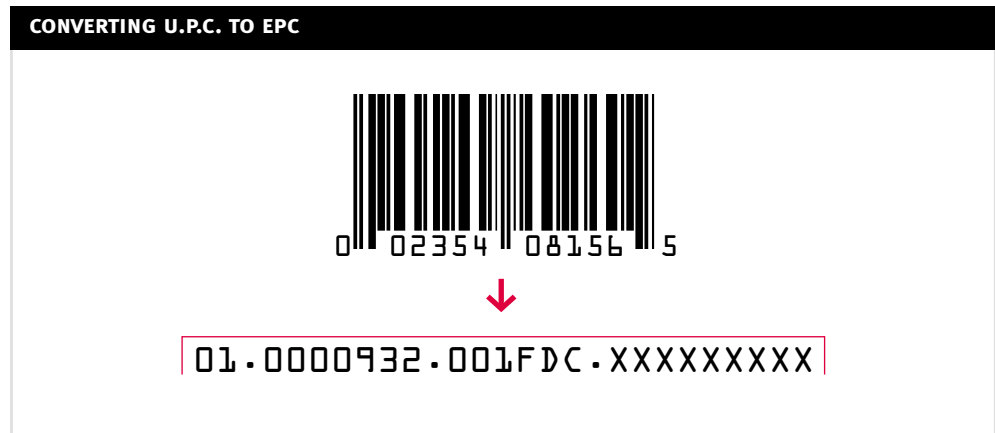
Figure B1. The manufacturer and item numbers of the U.P.C. code map directly into the manager and object class numbers of the EPC.
