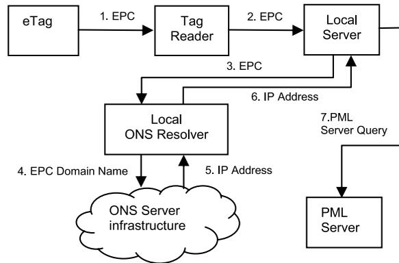
*Fig. 3: A tag reader detects the EPC stored in the electronic tag and retrieves the network IP address of the associated PML server through a query of the ONS resolver, which then directs the request to the authoritative ONS server.*
