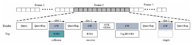
Figure 6: Multi-tag reply in EPC Class1 Gen.2 Protocol
