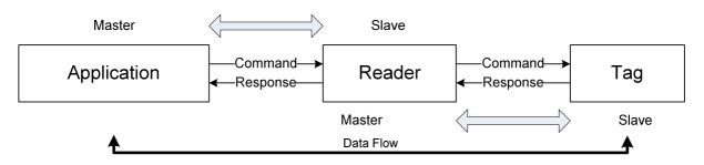
Figure 1: A Master-Slave Principle in RFID Systems
