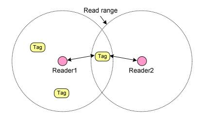
Figure 3: Reader-to-tag interference
