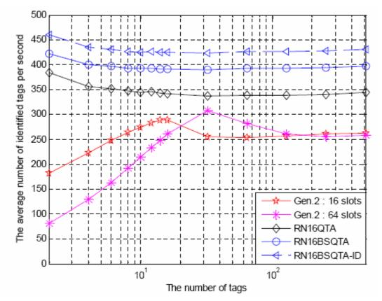
Figure 16: Identification Performance: RN16QTA and RN16BSQTA in Simple EPC Class 1 Gen.2 Protocol
