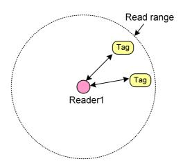
Figure 2: Tag-to-tag interference
