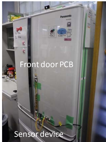
Figure 11 Sensor enabled refrigerator
