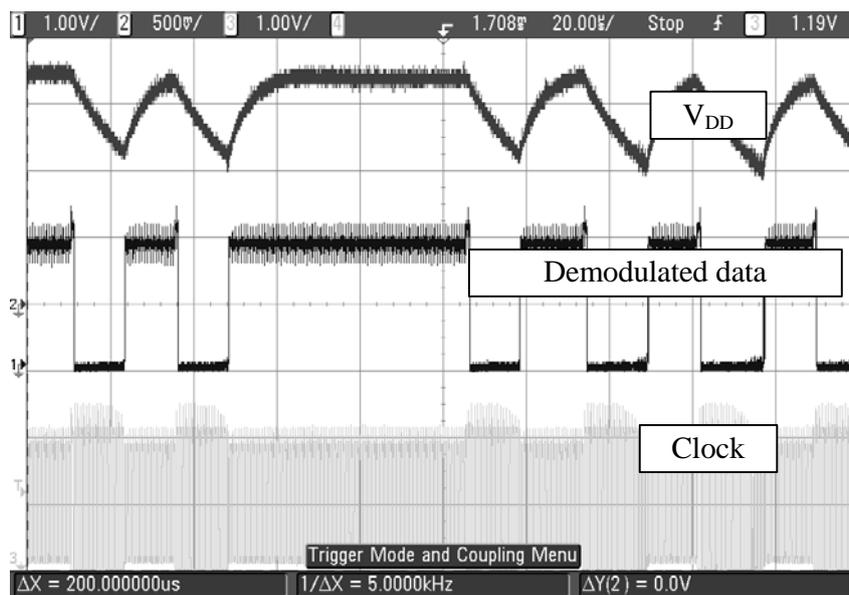
Fig.10 Rectified voltage, demodulated data and clock
