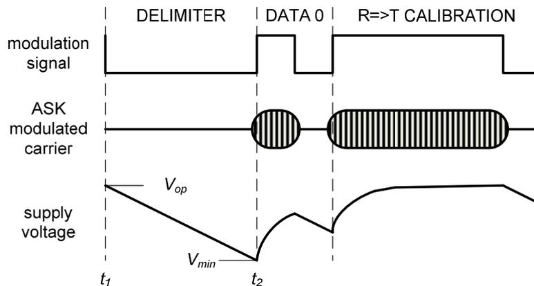
**Fig .2. Supply voltage's vs transmission signal**
