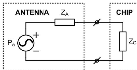
**Fig. 3 Equivalent model of the matching network**
