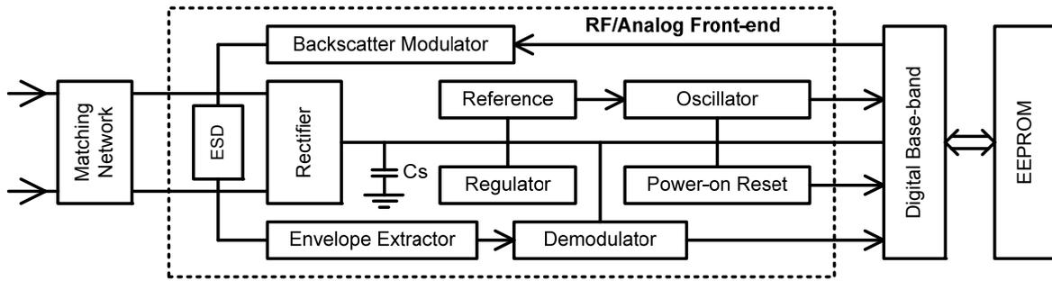
**Fig. 1. System architecture**
