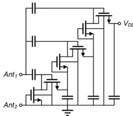
Fig. 4 Schematic of the AC-DC charge pump
