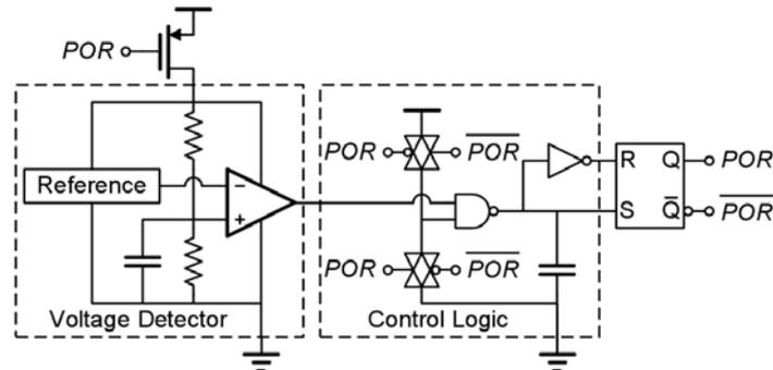
**Fig. 6. Schematic of the power-on reset circuit**
