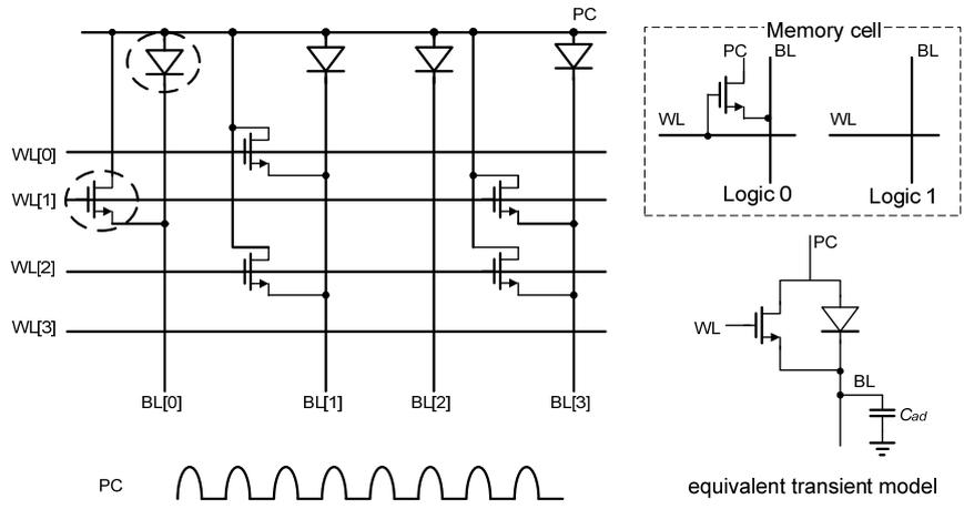
**Fig. 8: 4x4 ADL ROM and the equivalent transient model**
