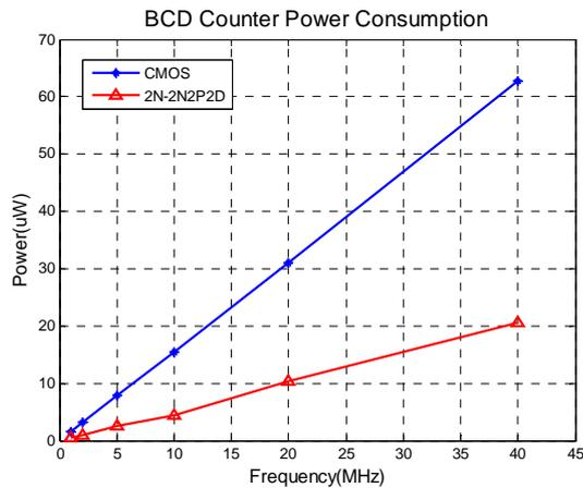
Fig. 7: Power dissipation of BCD counter built on CMOS & 2N-2N2P2D logic
