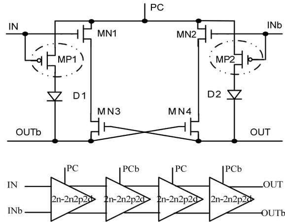
Fig. 6: Schematic of basic adiabatic 2N-2N2P2D logic gate
