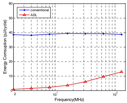
**Fig. 9: Power dissipation of Conventional & ADL ROM**
