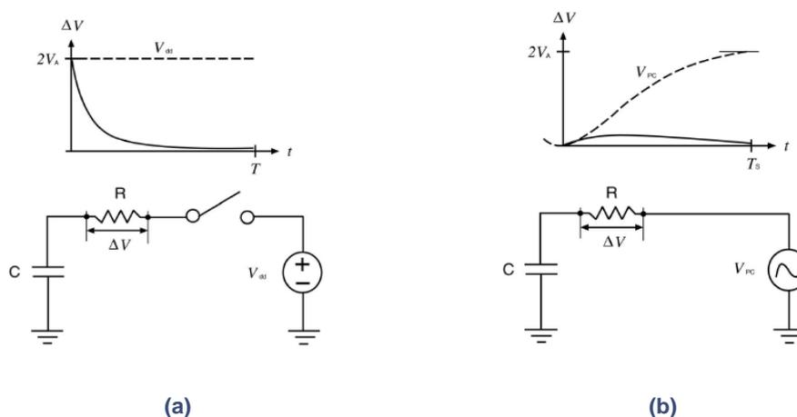
Fig. 1: Energy dissipation (a) CMOS circuit (b) Adiabatic circuit
