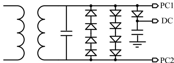
Fig. 5: Schematic of voltage limiter
