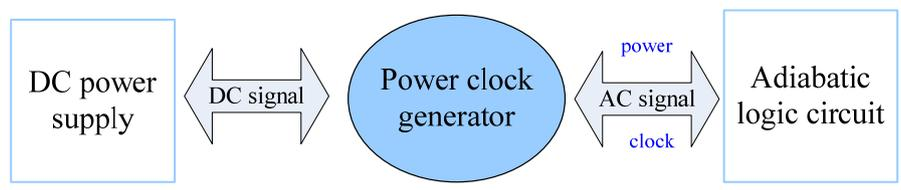
Fig. 2: Power supply scheme of adiabatic system
