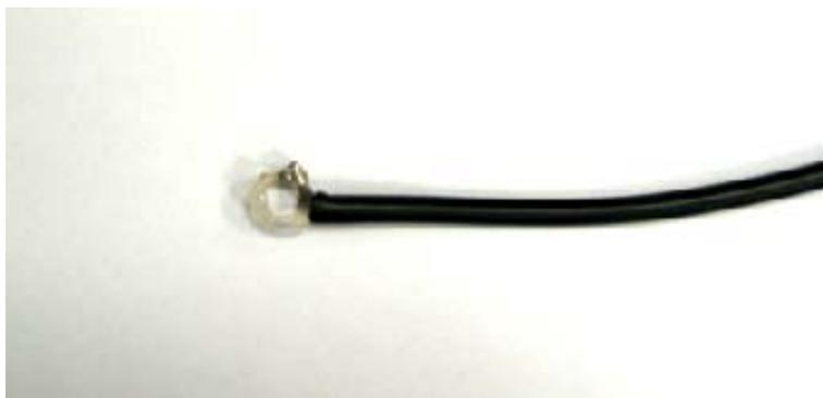
Figure 5: Small un-tuned loop
