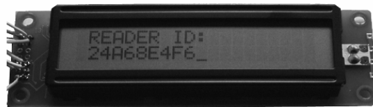
Figure 4: The display of the watchdog tag shows the decoded reader policy ID.
