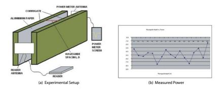
Figure 3: Waveguide: a packaging feature to improve tag readability
