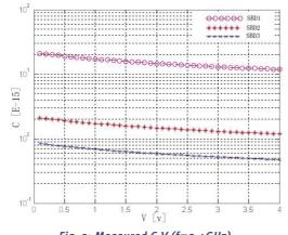
Fig. 5: Measured C-V (f=2.4GHz)
