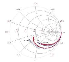
Fig. 11: Measurement and simulation S parameter of SBD1 from 50MHz to 40GHz(After de-embedding )
