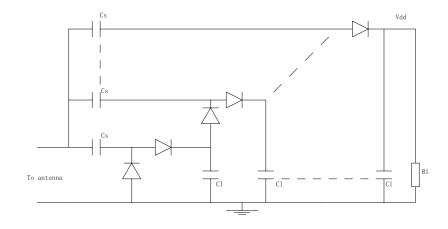
Fig. 12: Schematic of the rectify circuit use the voltage multiplier
