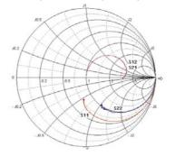
Fig. 7: Measurement S parameter of SBD1 from 50MHz to 40GHz (After de-embedding)
