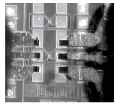
Fig. 8: Photo of realized SBD under probe measurement
