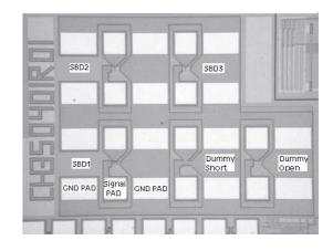
Fig. 6: Photo of SBDs and dummy with GSG probe pad
