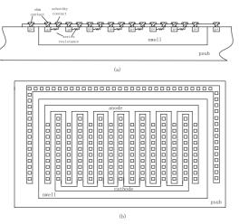
Fig. 2: (a) Cross section layout of realized Schottky diode. (b)Plane section layout of realized Schottky diode.
