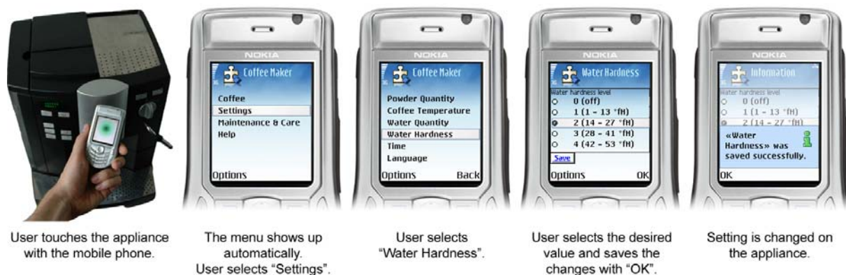
Fig. 4. Example of task solving using the AID. The water hardness can be changed more easily using the hierarchical menu of the AID, typically without consulting any manual.
