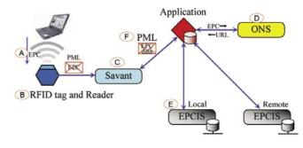
Fig. 1: Architecture of the EPC Network
