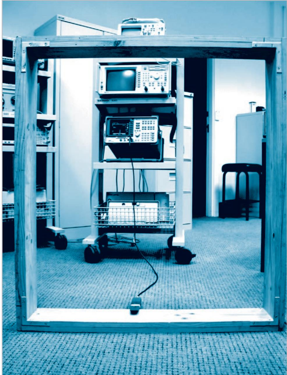
As just described, the large magnetic loop with the distributed capacitance should allow the current to be distributed more uniformly so that the assumption of uniform current distribution made in the analysis of physically small loop antennas is still true for physically large and no longer electrically small loop antennas.
