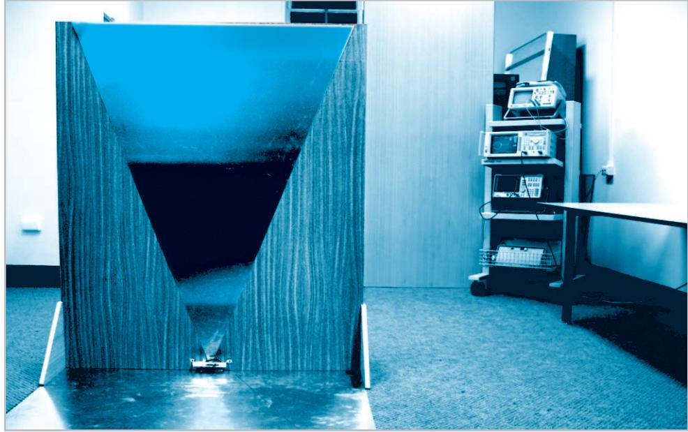
The model parameters for  $C_W$  and  $L_W$  can be conveniently obtained from the reactance  $X(\omega)$  plot of the monopole wedge above ground antenna. From the circuit model of Figure 2 the reactance is given by
