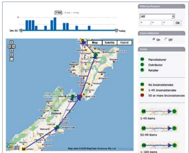
Figure 2. The Supply Chain Visualizer user interface. Green means no inconsistencies, yellow means that there are some inconsistencies but the number is below a predefined threshold, and red means that the number of inconsistencies at the particular node exceeds the threshold and thus indicates a serious problem.
